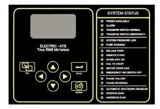
**Description** – Firetrol® Variable Speed Electric Fire Pump Controllers provide a variable frequency drive (VFD) in a PID process control loop to control the speed of a centrifugal pump for the purpose of limiting system pressure in a fire sprinkler system. These controllers are available in the following configurations:
